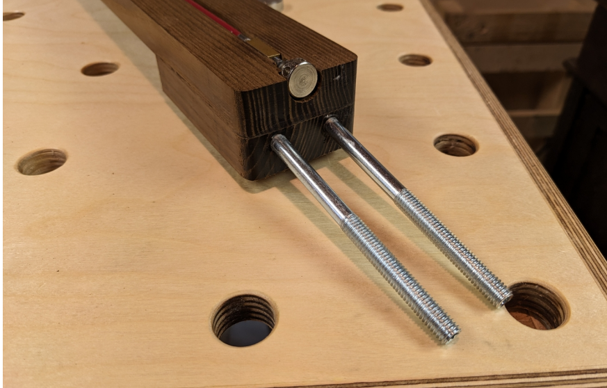
Figure 6: Inserted hanger bolts before being bent
